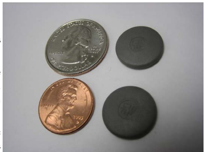
RFID chips are similar in size to coins
